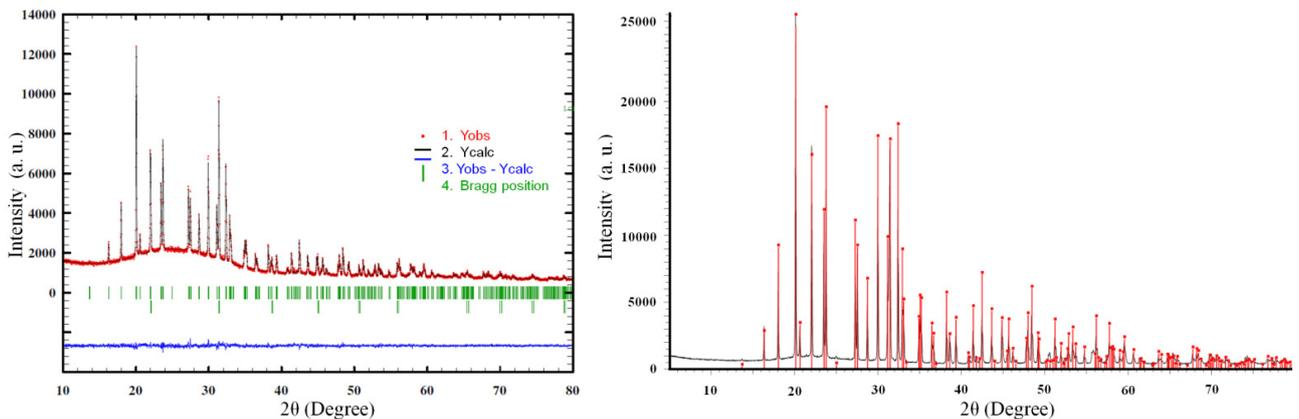
Fig. 6 XRD spectra of the LiBr/LiOH storage material before infiltration (on the left) and after infiltration into ZFT1700 Carbon felt (on the right).
