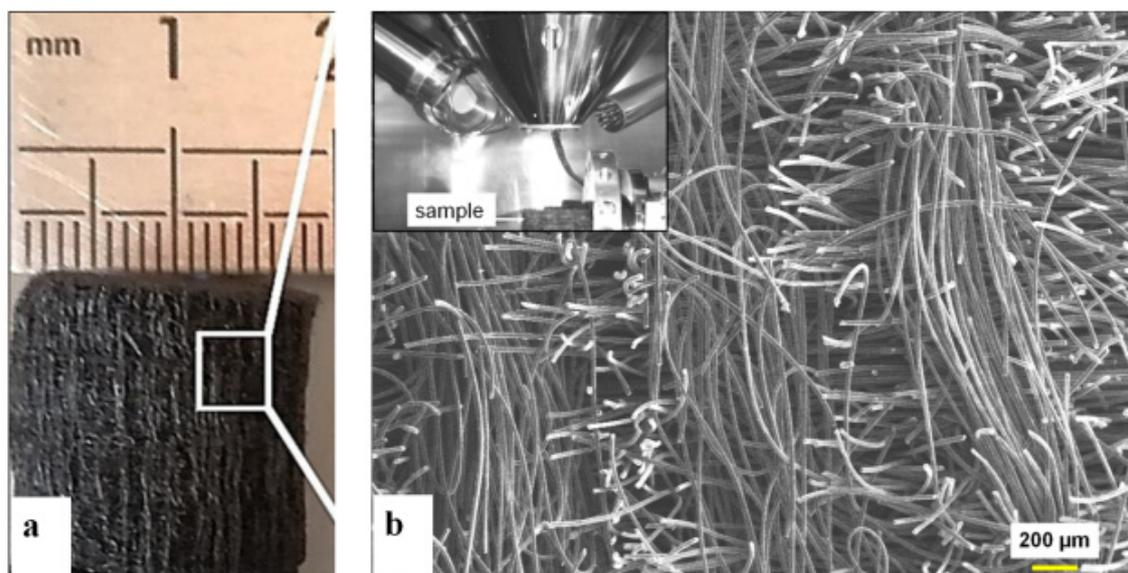
**Fig. 1** Optical pictures of ZFT1700 Carbon felt at (a) macroscopic and (b) microscopic scales (SEM picture).
