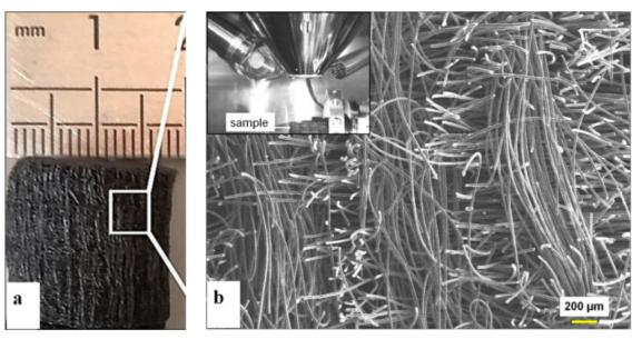
Fig. 1 Optical pictures of ZFT1700 Carbon felt at (a) macroscopic and (b) microscopic scales (SEM picture).
