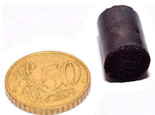
Figure 2. Typical cellular carbon monolith sample (here CRF450) obtained after pyrolysis and used as such for electrical conductivity and bulk density measurements.
