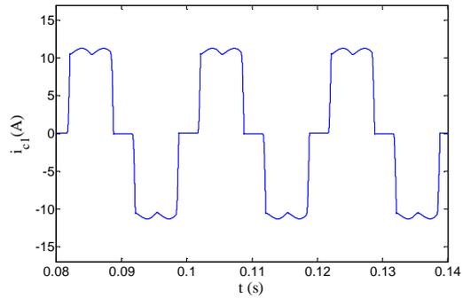
Fig. 14. Phase 1 source current without active filter.
