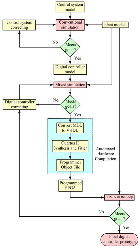
Fig. 2. System-level design flow.
