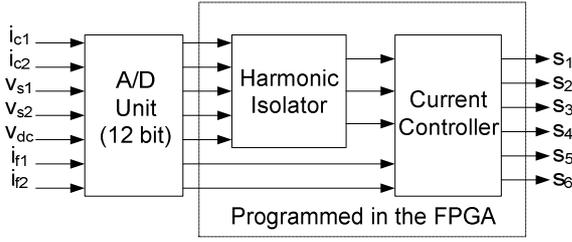
Fig. 7. Block diagram of the digital controller.
