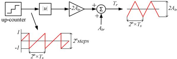
Fig. 12. Principle of the triangular carrier signal generator.
