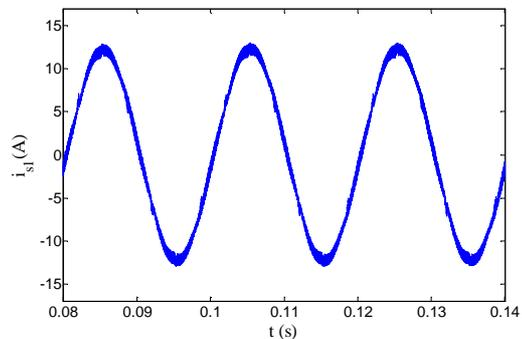
Fig. 16. Phase 1 source current with active filter.
