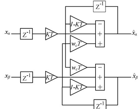
Fig. 9. Block diagram of the digital multi-variable filter.
