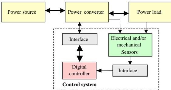
Fig. 1. Components of conventional power electronics systems.
