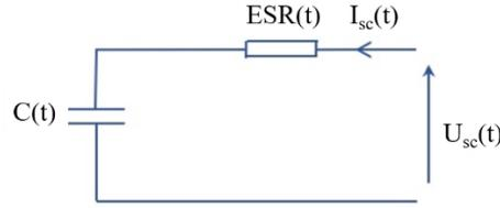
Figure 3. Thevenin electrical model of the SC.
