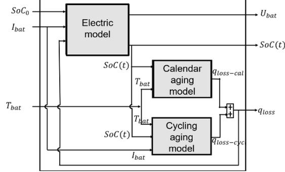
Figure 2. Electric and aging model of the battery.
