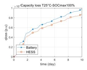
Figure 10. Battery capacity loss in HESS versus classical strategy 1.
