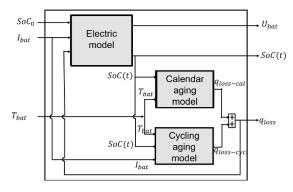
Figure 2. Electric and aging model of the battery.
