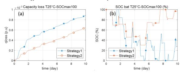
Figure 8. Capacity loss (a) and SOC of the battery (b) for strategies 1 and 2.
