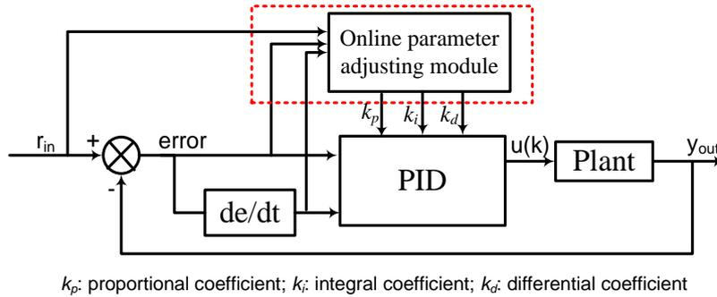
Figure 2: Schematic of the improved PID control system
