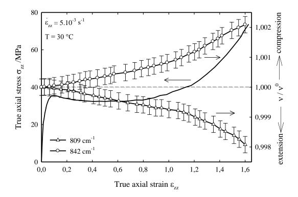
**Figure 8 :** Evolution of the true axial stress,  $\sigma_{zz}$ , and the normalized position,  $\nu / \nu^0$ , of amorphous band at 835 cm<sup>-1</sup> (C-C) in function of the true axial strain,  $\epsilon_{zz}$ , of iPP uniaxially stretched at T = 30 °C under a constant true strain rate  $\dot{\epsilon}_{zz} = 5.10^{-3} \, \mathrm{s}^{-1}$ .
