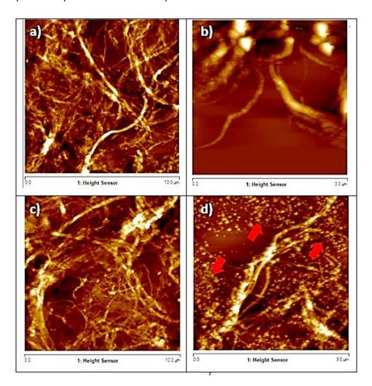
Figure 4: AFM height images of (a) WS-SC 10 μm x 10 μm, (b) WS-SC 3 μm x 3 μm, (c), WS-SteamEx 10 μm x 10 μm and (d) WS-SteamEx 3 μm x 3 μm. Lignin droplets are marked by red arrows in d. Key: WS, water swelling; SS, soda swelling; SC, soda cooking in autoclaves.
