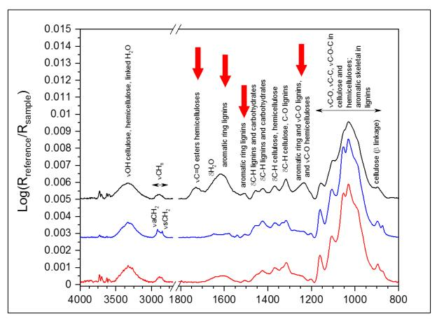
Figure 2: IR-ATR spectra of raw *Eucalyptus globulus* barks (dark), soda cooking in autoclave (red), and alkaline SteamEx (blue). Principal assignments are indicated. The spectra are normalized to one from region 1800-800 cm<sup>-1</sup>. For clarity, spectra were shifted vertically.
