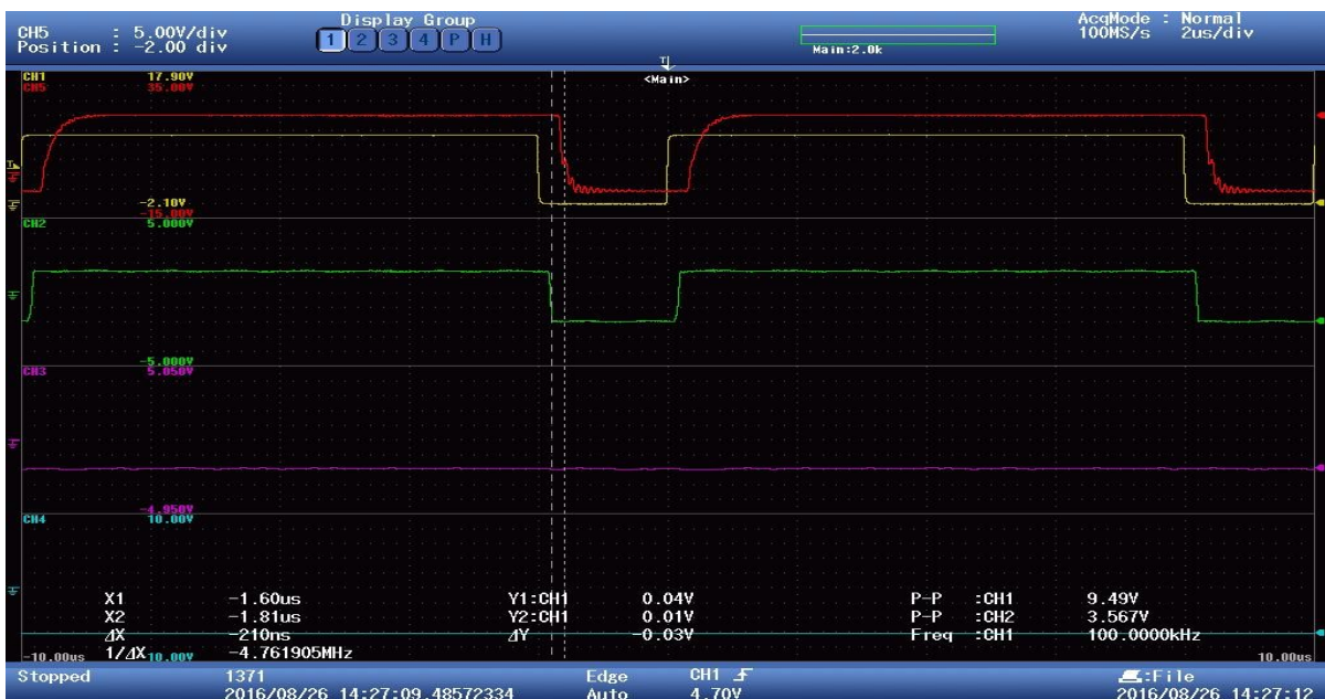
Figure 6.b) Driver card Prodrive® gate output Switching results up to 100 kHz
