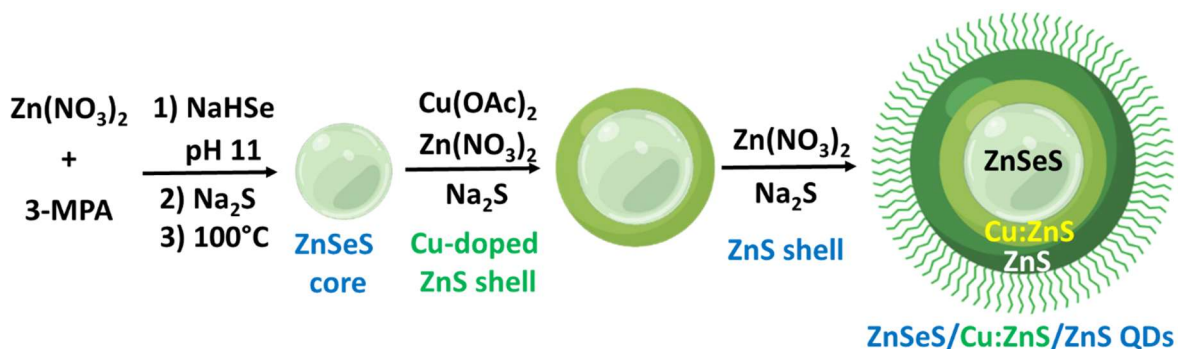
Scheme 1. Schematic representation of the synthesis of ZnSeS/Cu:ZnS/ZnS QDs.
