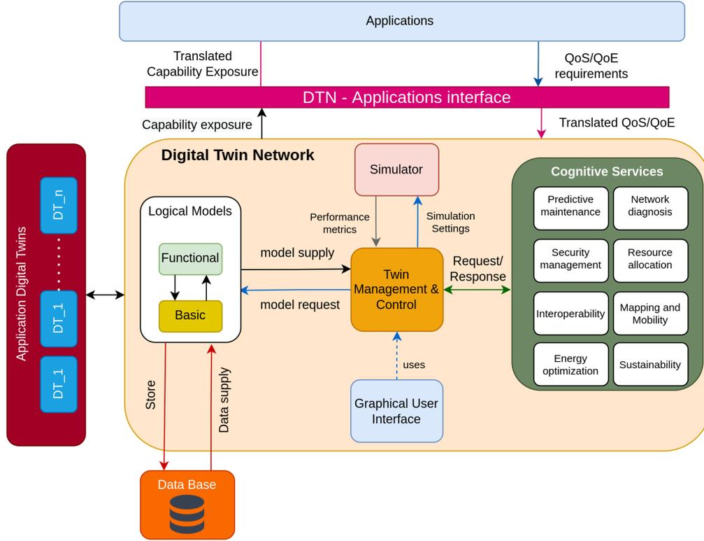
Fig. 2. Digital Twin Network internal architecture.
