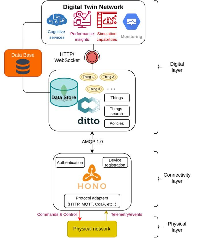
Fig. 1. Digital Twin Network using Eclipse Ditto + Hono.
