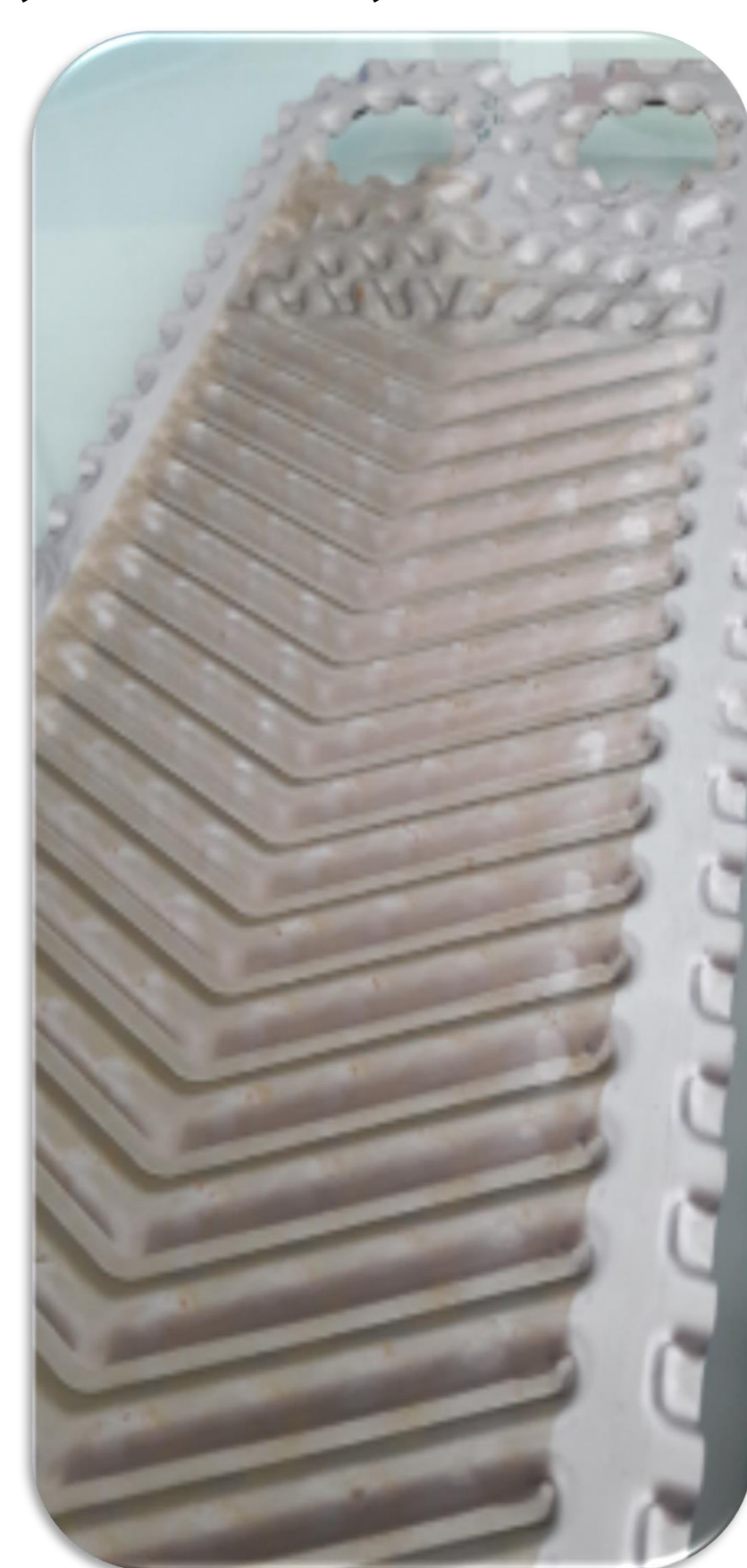
Stainless steel plate (cm) (length 42; width 12; thickness 0.06)
