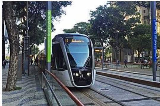
Energy recovery - SC equipped tram, Rio Janeiro Light Rail
