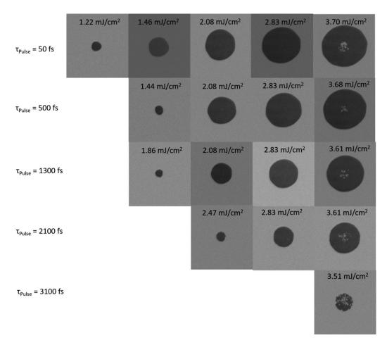
FIG. 1. Magneto-optical images of  $Gd_{15.9}Tb_{6.1}Co_{78}$  after exposure to a single linearly polarized laser pulse with a pulse duration of 50, 500, 1300, 2100, and 3100 fs, and with various fluences ranging from 1.22 to 3.7 mJ/cm<sup>2</sup>.
