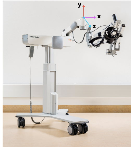
Figure 1: The Armeo Spring device, a passive orthotic exoskeleton for upper limb rehabilitation training. The reference frame attached to the shoulder sensor defines all the positional measurements recorded in the dataset used for our study. The image is courtesy of Hocoma Inc. Switzerland.
