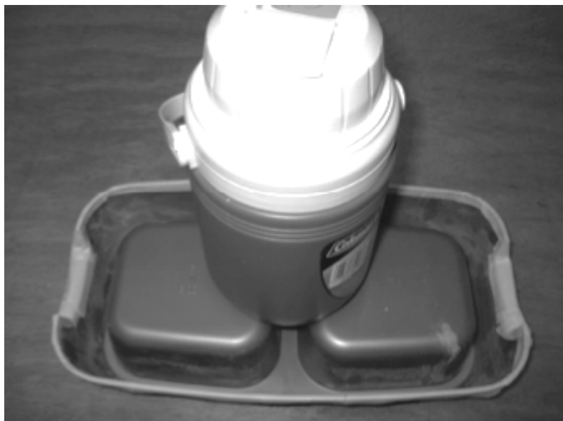
FIGURE 46 : PIEGE FAIT MAISON A BASE DE GLACE SECHE (WANG ET AL, BED BUG ATTRACTION TO PITFALL TRAPS BAITED WITH CARBON DIOXIDE, HEAT, AND CHEMICAL LURE. JOURNAL OF ECONOMIC ENTOMOLOGY,2009)
