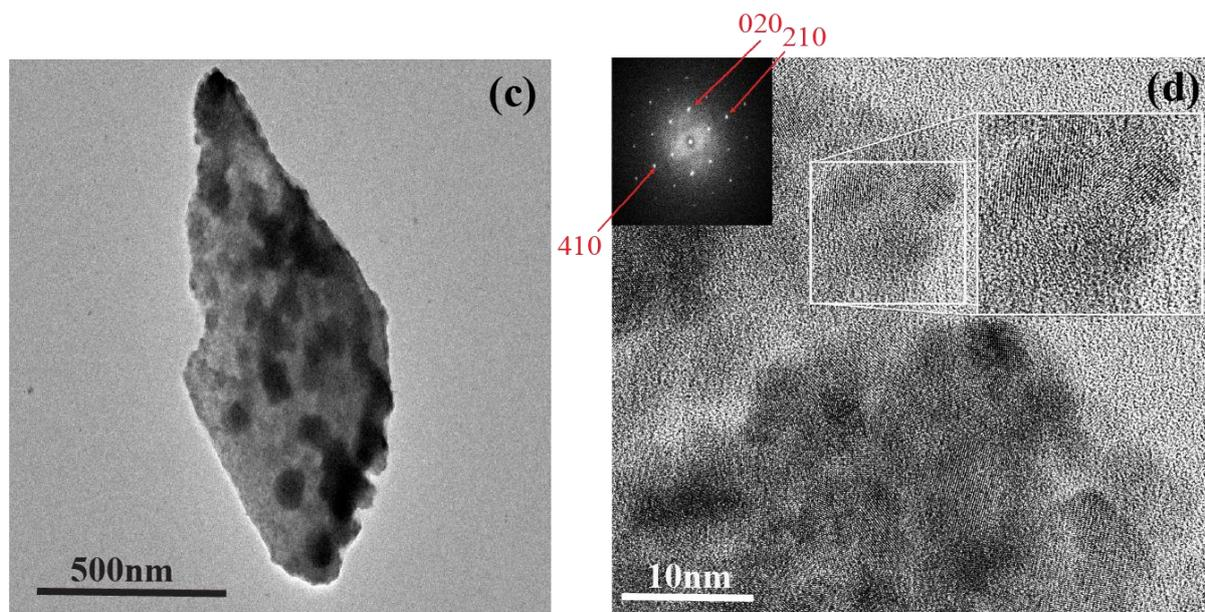
**Figure 5.** Representative TEM and HRTEM images and corresponding FFT patterns of BaSO<sub>4</sub> formed at the interface of Ba<sup>2+</sup> in the organic phase and SO<sub>4</sub><sup>2-</sup> in the aqueous phase (a,b) or Ba<sup>2+</sup> in the aqueous solution and HSO<sub>4</sub><sup>-</sup> in the organic phase (c,d).
