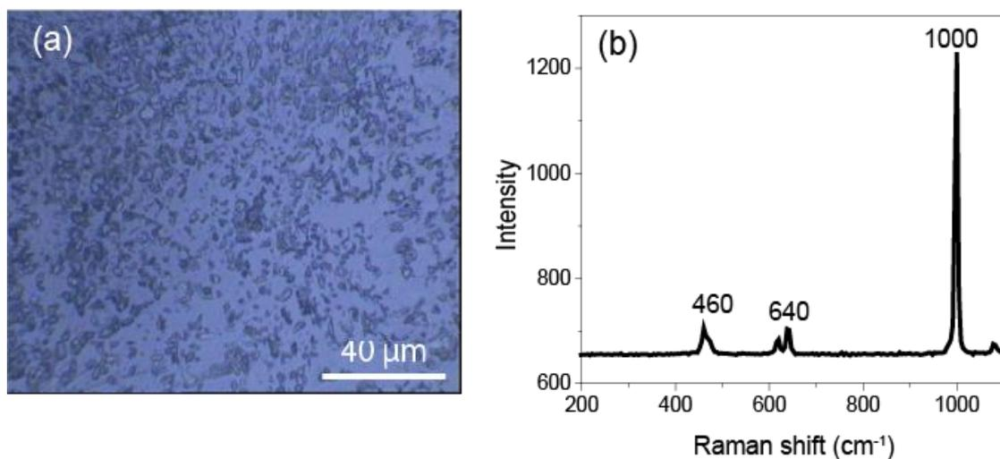
**Figure 2.** Confocal Raman microscopy and spectroscopic characterisation. (a) Optical image of BaSO<sub>4</sub> formed at the glass capillary mouth, (b) Raman spectrum of the observed crystals.
