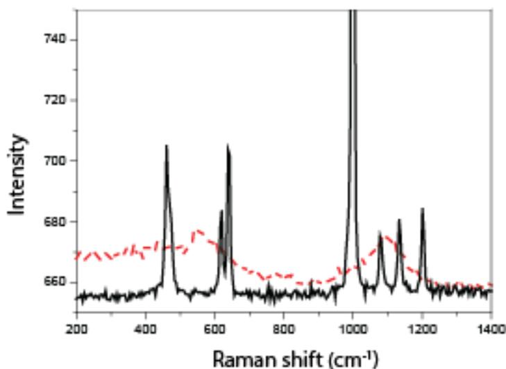
**Figure 6.** Raman spectra for  $\text{BaSO}_4$  crystallisation, in the absence of organic phase ionophore (solid line) and in the presence of organic phase ionophore (dashed line), indicating no formation of  $\text{BaSO}_4$  in the latter. Raman spectra were taken from the mouth of the capillary in each case.
