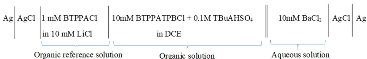
**Scheme 2.** Electrochemical cell composition used in investigating crystallisation following spontaneous transfer of hydrogen sulfate ions from organic to aqueous phase to form barium sulfate crystals.
