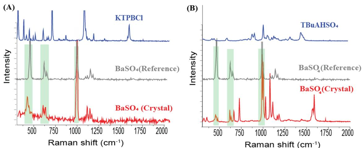
**Figure 3.** Raman spectra for BaSO<sub>4</sub> crystallisation at the ITIES: (A) formed between organic solution of Ba(TPBCl)<sub>2</sub> and aqueous solution of SO<sub>4</sub><sup>2-</sup> (Scheme 1); (B) formed between aqueous solution of Ba<sup>2+</sup> ions and organic solution of TBuAHSO<sub>4</sub> (Scheme 2). KTPBCl is potassium tetrakis(4-chlorophenyl)borate. TBuAHSO<sub>4</sub> is tetrabutylammonium hydrogensulfate. Reference indicates the spectrum of commercially-available material.
