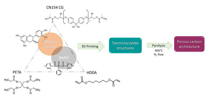
Figure 1. Scheme of the synthesis method of 3D-printed tannin-based carbon architectures.
