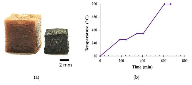
**Figure 2.** (a) Example of 3D-printed structures before (**left**) and after pyrolysis (**right**). (b) Heating ramp for the pyrolysis step.
