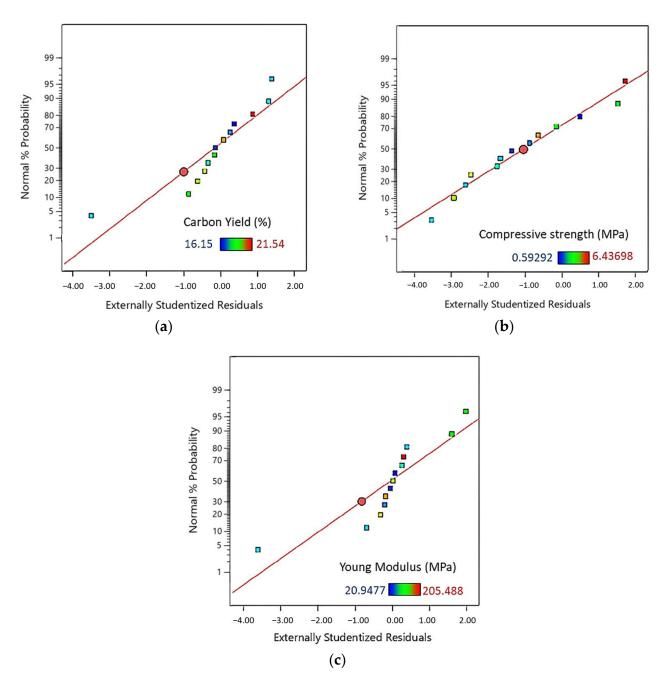
**Figure 6.** Normal probability plot for residuals for: the (a) carbon yield, (b) compressive strength, and (c) Young's modulus. The numerical values for these properties increase from dark blue to red.
