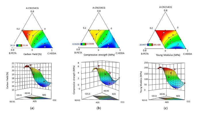
**Figure 7.** Contour plots (**top**) and surface plots (**bottom**) of the effect of the acrylate ratio on: the (**a**) carbon yield, (**b**) compressive strength, and (**c**) Young's modulus. The numerical values of the responses increase from dark blue to red.
