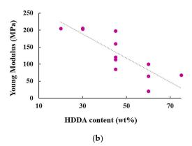
**Figure 5.** (a) Stress–strain curves of some 3D-printed carbon studied in this work. (b) Young modulus as a function of the initial HDDA content.
