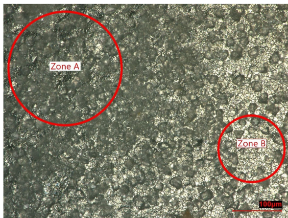
Figure 15. Distribution of calcium carbonate in the middle of the first compartment after 3 days of operation at magnification ( \times 500 ).
