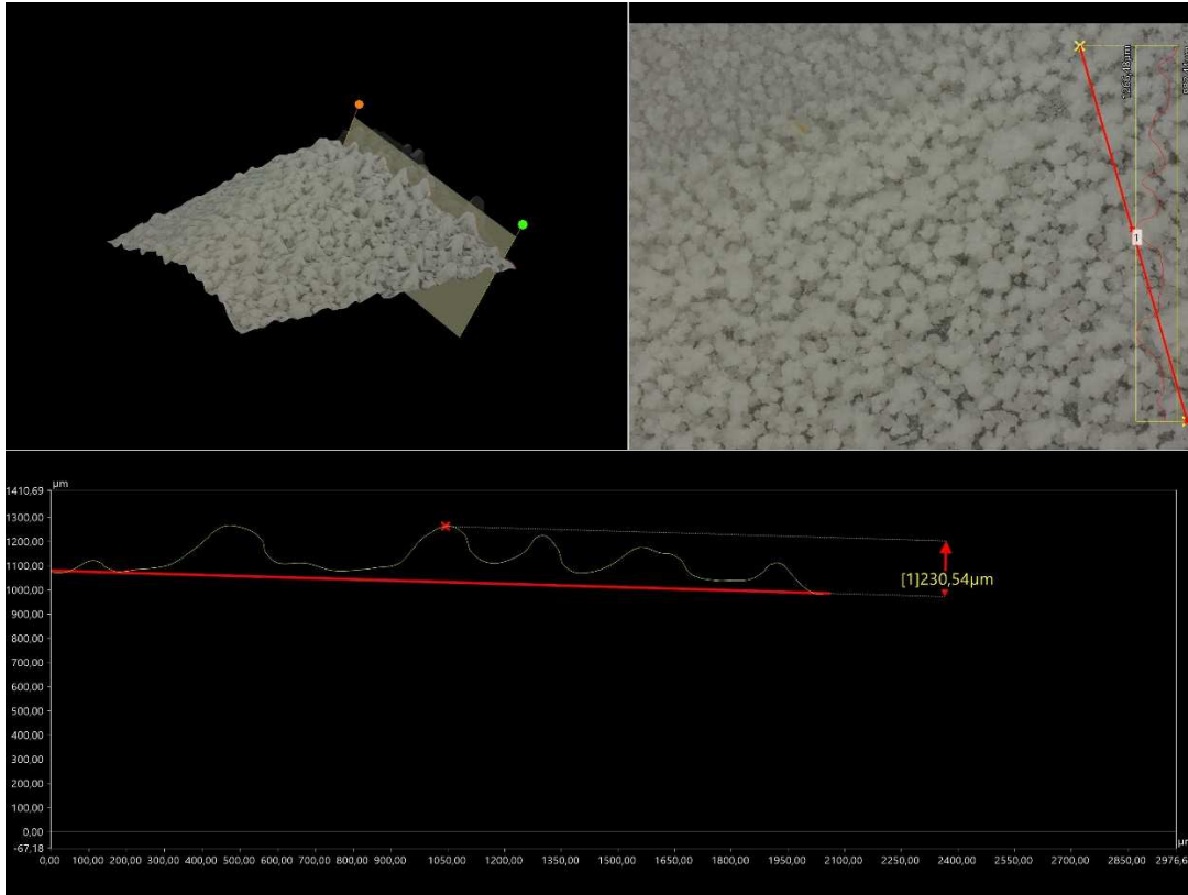
Figure 7: Results of digital microscope 3D - the thickness of the deposited scale in the inlet of the first cold compartment without treatment after 72 hours of heating, 50 °C, 100 L.h -1
