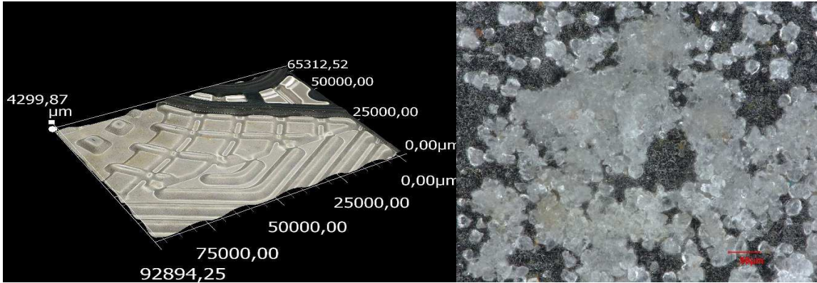
Figure 6: Scale crystals deposited on the 316L steel exchanger plate at the inlet and outlet of the first cold compartment scanned by the 3D digital microscope after 72 hours of operation, 50 °C, 100 L.h -1
