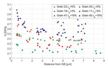
Fig. 6. Nanohardness H as a function of the distance from GB for the undeformed sample in grains 22 and 20; the deformed samples at  $\epsilon_{\rm p}=3\%$  in grains 11 and 19, and, at  $\epsilon_{\rm p}=18\%$  in grains 47 and 40.
