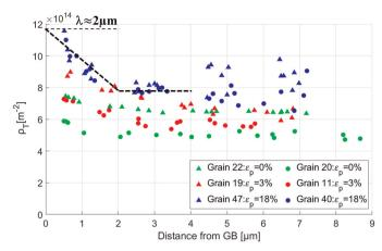
Fig. 7. Total dislocation density  $\rho_T$  estimated from H as a function of the distance from GB for the undeformed sample in grains 22 and 20; the deformed samples at  $\varepsilon_p = 3\%$  in grains 11 and 19, and, at  $\varepsilon_p = 18\%$  in grains 47 and 40. The black dotted lines are a guide for the eye to estimate the thickness  $\lambda$  of the grain boundary affected layer.
