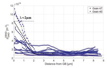
Fig. 5. Moving average with n = 15 of GND density measured by EBSD of specimens deformed at  $\varepsilon_{\rm p} = 18\%$  for grains 40 and 47. The red line represents the noise threshold of GND density,  $\rho_{GND}^{noisethsd} = 7.0 \times 10^{13} m^{-2}$ . The black dotted lines are a guide for the eye to estimate the thickness  $\lambda$  of the grain boundary affected layer.
