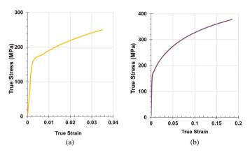
Fig. 1. True stress-strain curves of Al-k ferritic steel of both tensile specimens loaded up to respective plastic strains: (a)  $\varepsilon_{\rm p} = 3\%$  and (b)  $\varepsilon_{\rm p} = 18\%$ .
