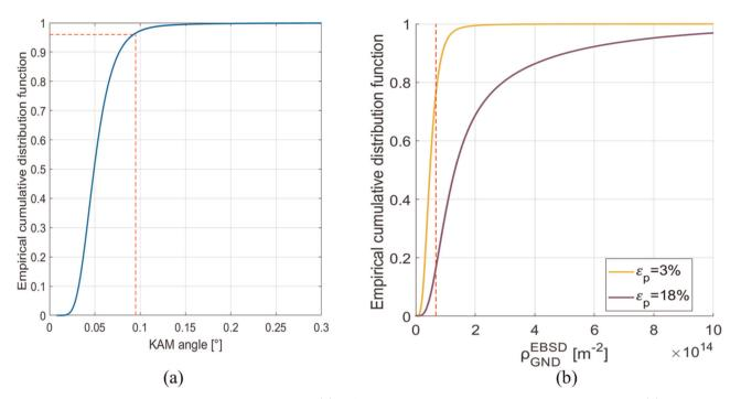
Fig. 3. Empirical cumulative distribution function of (a) KAM angle for undeformed Al-killed ferritic steel, (b) GND density determined by EBSD for 3% and 18% plastic strains, respectively.
