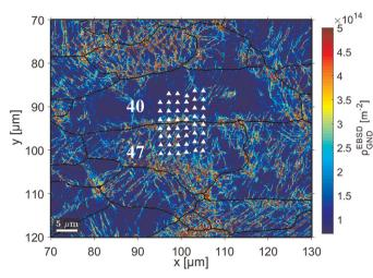
Fig. 4. GND density map of the Al-k specimen deformed at  $\varepsilon_{\rm p} = 18\%$ . Indents in grains 40 and 47 are also reported (see Fig. 2c).
