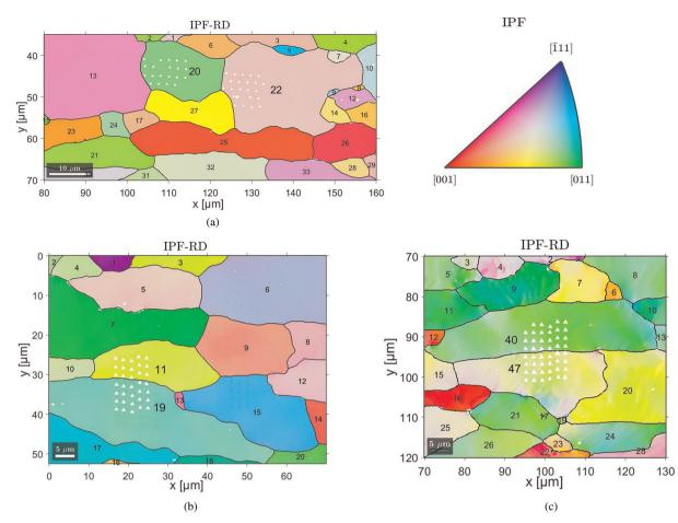
Fig. 2. Inverse pole figures along the RD direction of the undeformed specimen (a), the deformed specimen at 3% (b) and 18% (c) plastic strains, respectively. The indent locations are also reported at each plastic strain level.
