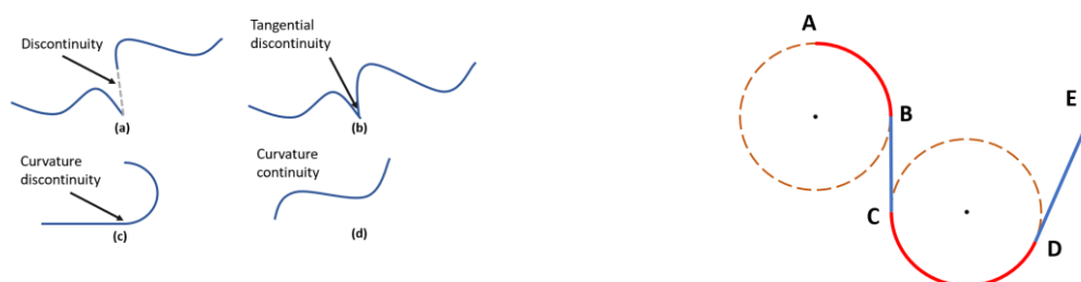
Figure 2 Parametric continuity paths. (a) Discontinuous segments. (b) C^0 continuity. (c) C^1 continuity. (d) C^2 continuity.
