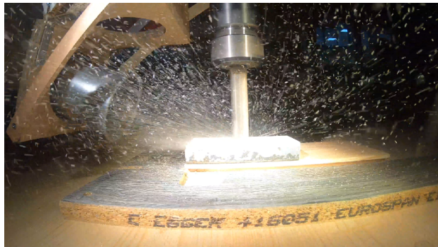
Fig. 1: Picture of wood dust emission during the robotic grooving. We constructed an experimental setup composed of an industrial gantry robot to understand how dust particles are emitted for operational conditions such as feed speed and rotational speed.
