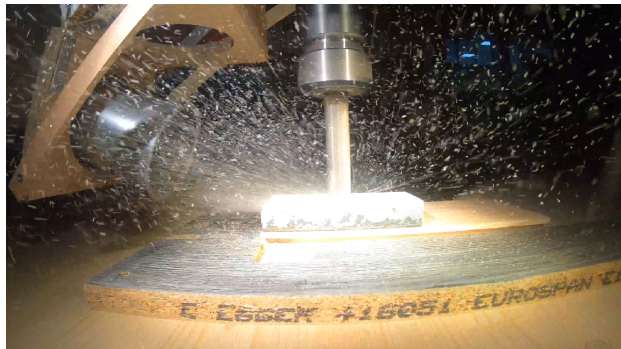
Fig. 1: Picture of wood dust emission during the robotic grooving. We constructed an experimental setup composed of an industrial gantry robot to understand how dust particles are emitted for operational conditions such as feed speed and rotational speed.
