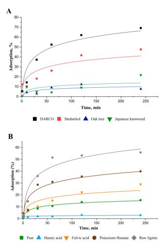
Fig. 2. Effect of contact time on  $\alpha$ -HCH adsorption on activated carbons and biochars (Fig. 2A) and on soil organic matter (Fig. 2B). Pesticide and sequestrant concentrations were 50 µg/L and 0.13 g/L, respectively. Results based on 2 replicates.
