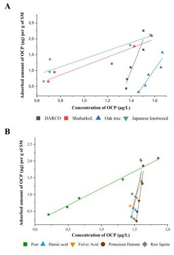
Fig. 4. Freundlich adsorption isotherms of  $\gamma$ -HCH and studied activated carbons and biochars (Fig. 4A) and soil organic matters (Fig. 4B). Working conditions: Contact time 48 h, temperature 25 °C, agitation 150 rpm, initial OCP concentration 50 µg/L, SM concentrations: 0.1. 0.4. 2.0. 5.0. 10 g/L.
