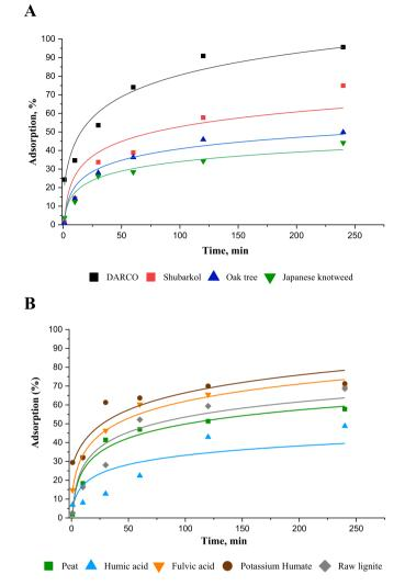
Fig. 1. Effect of contact time on 4,4-DDT adsorption on activated carbons and biochars (Fig. 1A) and on soil organic matter (Fig.1B). Pesticide and sequestrant concentrations were 50  $\mu$ g/L and 0.13 g/L, respectively. Results based on 2 replicates.
