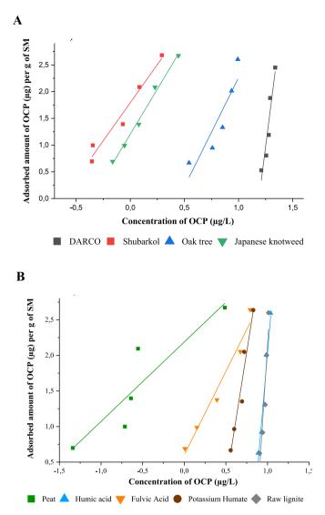
Fig. 3. Freundlich adsorption isotherms of 4,4-DDE and studied activated carbons and biochars (Fig. 3A) and soil organic matters (Fig. 3B). Working conditions: Contact time 48 h, temperature 25 °C, agitation 150 rpm, initial OCP concentration 50  $\mu$ g/L, SM concentrations: 0.1. 0.4. 2.0. 5.0. 10 g/L.
