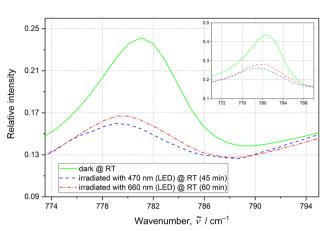
Fig. 3 The  $781\,\mathrm{cm}^{-1}$  IR band, attributed to the  $\delta(\mathrm{NO_2})$  scissoring vibration, indicating switching. The RT spectra are recorded before any irradiation (green solid line), after 470 nm LED irradiation (blue dashed line) and after final 660 nm LED irradiation (red dotted–dashed line). The inset plot shows the same peak and its behaviour when irradiated with the 476 nm laser light (1 h), and then with the 556 nm laser light (1.5 h).
