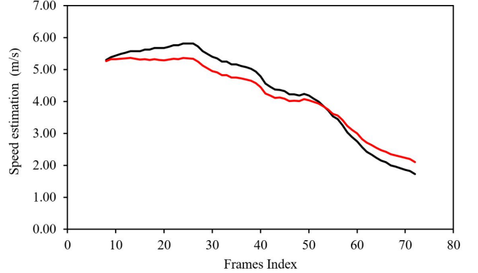
Fig. 8. Real speed estimation. Black: the linear projection model, Red: the equidistant projection model.
