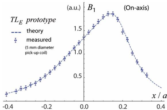
Fig. 11. Measured profile of the on-axis magnetic field produced by the  $TL_E$  three-coil prototype. Measurements were carried out in free space using the pick-up coil described in the text. Dashed line represents the normalized theoretical curve (see Fig. 4b).
