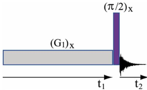
Fig. 13. Basic sequence for a two-dimensional experiment involving a  $B_1$  gradient ( $G_1$ ). Phases of the  $B_1$  gradient pulse and of the  $\pi/2$  pulse (optional) must be identical.  $t_1$  is incremented so as to form a 2D map ( $t_1, t_2$ ) which is further subjected to a double Fourier transform. This pulse leads to a cosine modulation in the spatial dimension (perhaps more convenient for data treatment). Without it, one would have a sine modulation.
