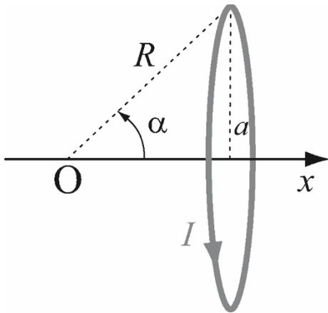
Fig. 1. Geometry of a general current loop carrying a current  $I$ , with radius  $a$  and symmetry axis  $Ox$  (at a radial distance  $R$  from the origin and subtending an angle  $\alpha$  with  $x$ -axis).
