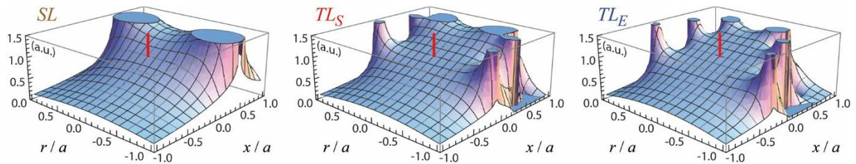
Fig. 5. 3D representation, corresponding to a  $rx$ -plane (any plane containing the symmetry axis  $x$ ), of the axial component  $B_{1x}$  of the magnetic field produced by the coil systems (see text): configurations  $TL_S$ ,  $TL_E$  and  $SL$ . Position of the origin  $O$  is marked by a centered vertical line (in red). For all configurations, the outer coil has the same radius  $a$ . The three coil systems are assumed to be driven by the same current  $I$ .
