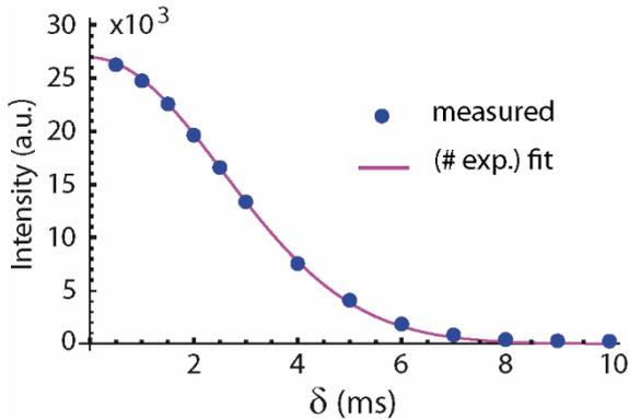
Fig. 12. A typical diffusion experiment performed on a water sample with the  $B_1$  gradient system described above. The horizontal scale corresponds to the  $\delta$  values in ms.  $\Delta$  is set to 0.4 s. The dead time of the three-coil system is about  $6.5 \mu\text{s}$ , and the RF amplifier power used for the experiments was about 150 W. With a diffusion coefficient of  $2 \cdot 10^{-5} \text{ cm}^2\text{s}^{-1}$ , we obtain a
