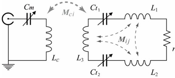
Fig. 9. Equivalent circuit model of the gradient three-coil system with its self-inductances  $L_i$  ( $i = 1,2,3$ ), the mutual inductances  $M_{ij}$  ( $i \neq j = 1,2,3$ ) and its symmetric tuning capacitors  $Ct_1$  and  $Ct_2$ . The resistor  $r$  accounts for losses in the gradient coil system. Matching is achieved by a moveable tuned coupling loop. Both primary and secondary circuits are tuned to the Larmor frequency. Magnetic couplings are indicated by dashed lines.
