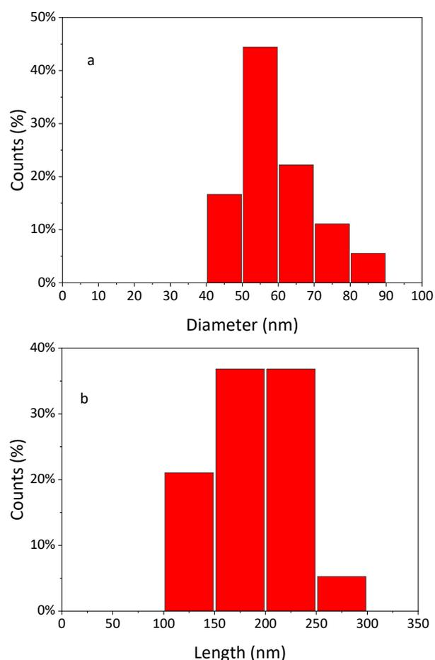
Fig. 3: a) Diameter and b) Length of Te nanorods deposited at  $C_1$  peak potential in EOipTFSI:EOipBr 95:5 (mol%).  $[\text{TeCl}_4] = 5 \text{ mM}$ .  $T = 100 \text{ }^\circ\text{C}$ ,  $Q = 0.1 \text{ C/cm}^2$  (number of analyzed nanowires  $n = 18$ ).
