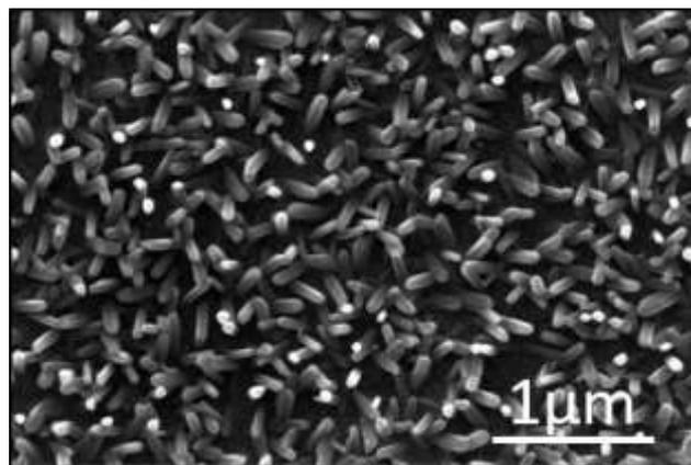
Fig. 2: SEM image of Te nanorods electrodeposited at  $C_1$  peak potential in EOipTFSI:EOipBr 95:5 (mol%).  $[\text{TeCl}_4] = 5 \text{ mM}$ .  $T = 100 \text{ }^\circ\text{C}$ ,  $Q = 0.1 \text{ C/cm}^2$ , Pt-coated glass slide.
