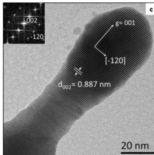
Fig. 9: TEM characterization of stützite nanorods after 6h immersion, prepared with  $n\text{Ag(I)}/n\text{Te} = 2$ : a) TEM image of a stützite slightly curved nanorods group, b) TEM image of diameter-enhanced stützite nanorod, c) corresponding HRTEM micrograph and Fast Fourier Transform (FFT) of stützite crystallographic structure along the [210] zone axis (SG: P-62m) (JCPDS n° 04-008-4552).
