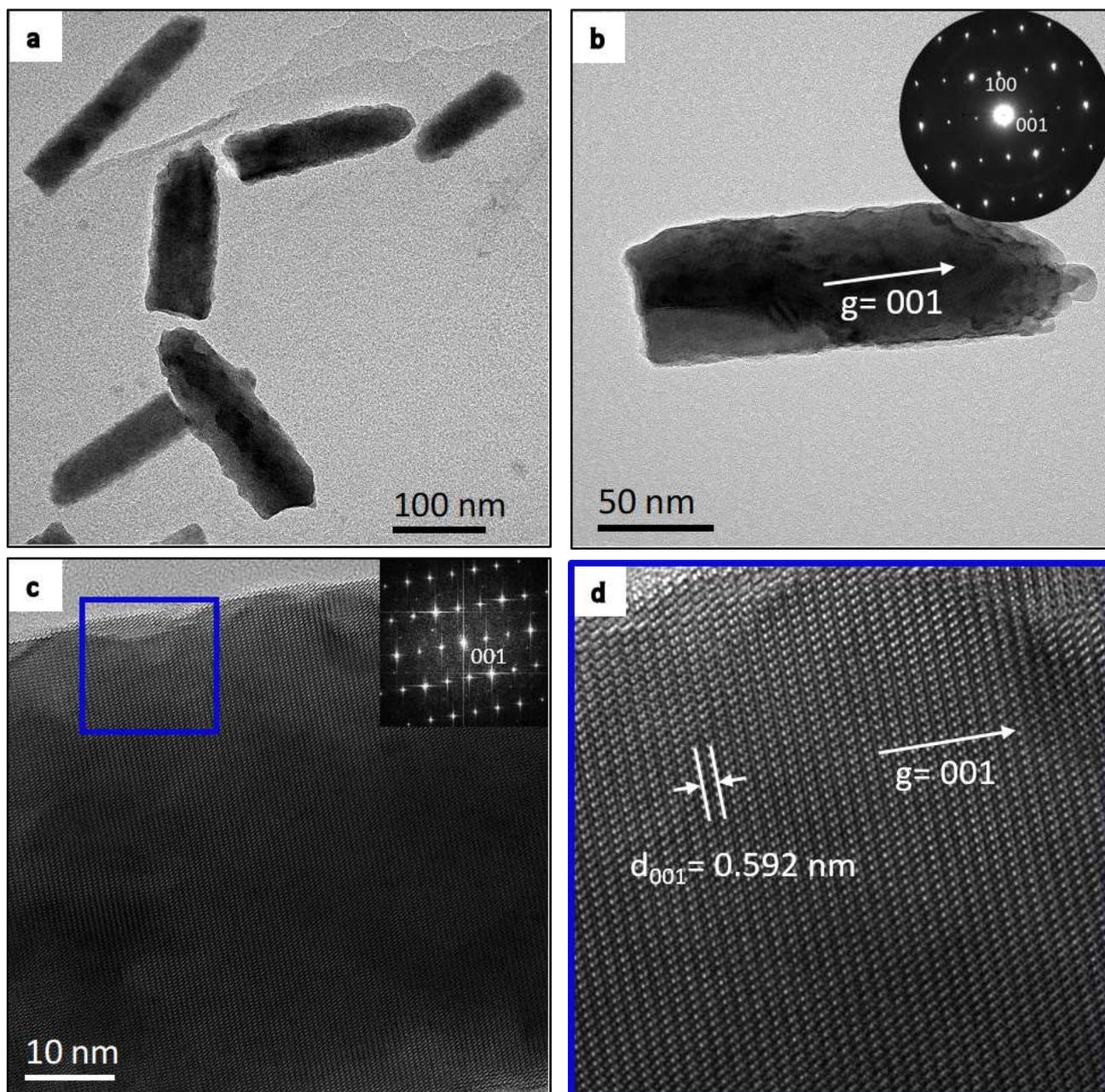
Fig. 4: TEM characterization of Te nanorods: a) TEM image of a Te nanorods group, b) TEM micrograph and corresponding SAED pattern indexed to the tellurium phase along the [010] zone axis (SG: P3<sub>1</sub>21), c) HRTEM micrograph with Fast Fourier Transform (FFT) and d) Zoom on the blue square of Te crystallographic structure along the [010] zone axis (JCPDS n° 00-036-1452).
