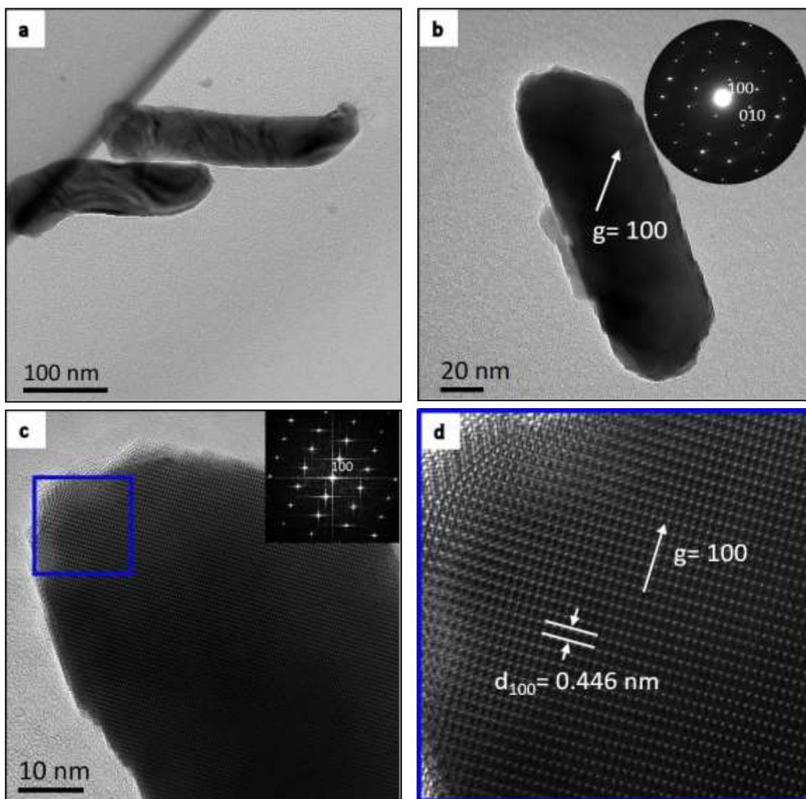
Fig. 12: TEM characterization of hessite nanorods after 24h immersion prepared with  $n\text{Ag(I)}/n\text{Te} = 2$ : a) TEM image of a  $\text{Ag}_2\text{Te}$  nanorods group, b) TEM micrograph and corresponding SAED pattern indexed to the hessite phase along the [001] zone axis (SG:  $P12_1/C1$ ), c) HRTEM micrograph with Fast Fourier Transform (FFT) and d) Zoom on the blue square of  $\text{Ag}_2\text{Te}$  crystallographic structure along the [001] zone axis (JCPDS n° 01-081-1820).
