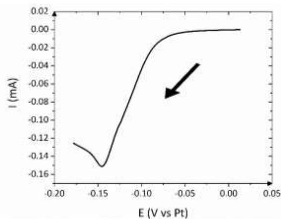
Fig. 1: Typical linear sweep voltammogram of the reduction of Te(IV) to Te(0) in EOPipTFSI:EOPipBr 95:5 (mol%). [TeCl<sub>4</sub>] = 5 mM. Pt-coated glass slide substrate. T = 100 °C, scan rate 5 mV s<sup>-1</sup>.
