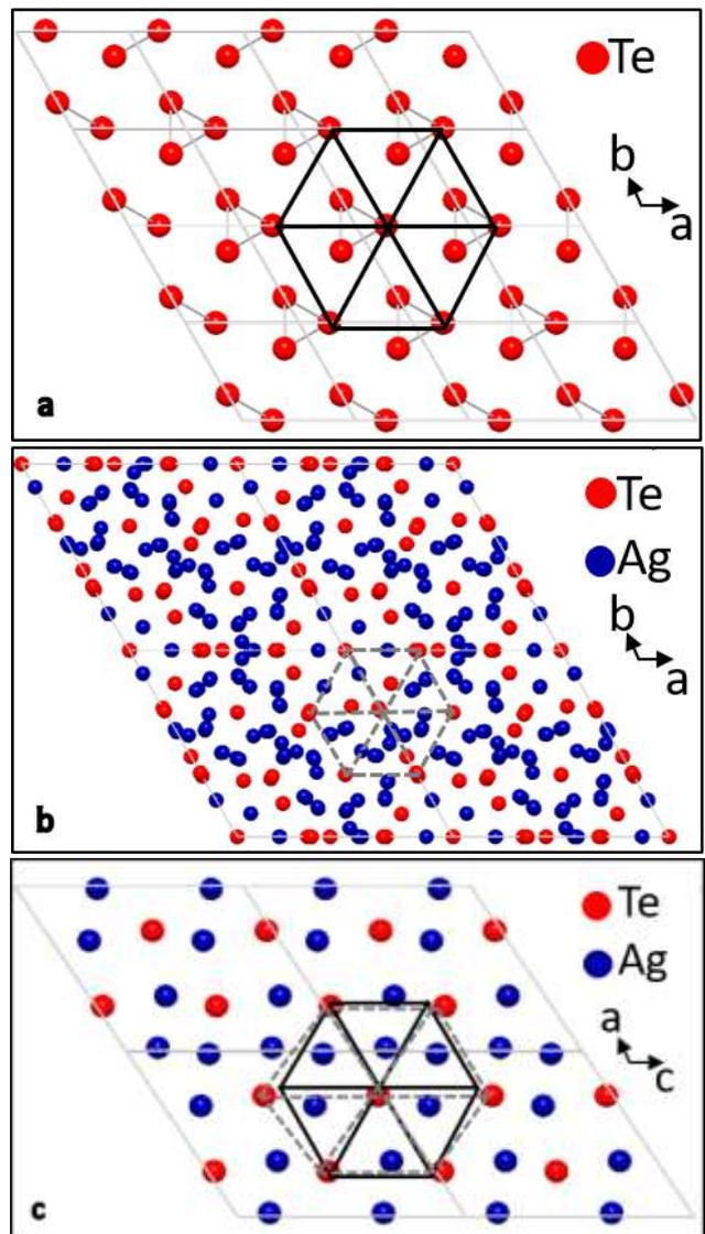
Fig. 15: Crystalline structure of a) Hexagonal Te; b) Hexagonal stutzite; c) Monoclinic hessite.
