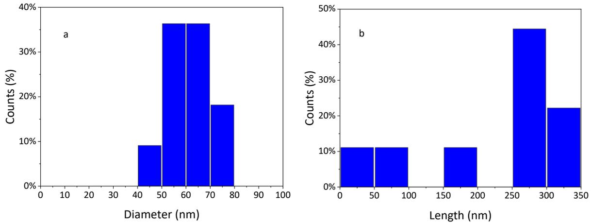
Fig. 13: a) Mean diameter and b) Length of hessite nanorods after 24h immersion prepared with  $n\text{Ag(I)}/n\text{Te} = 2$  (number of analyzed nanowires  $n = 9$ ).
