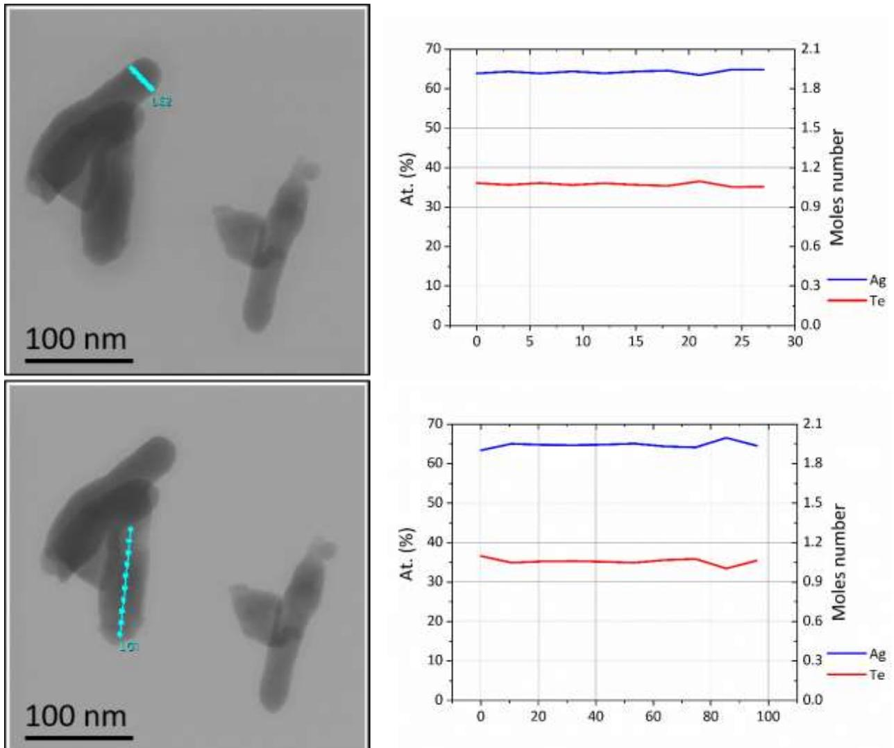
Fig. 10: Line profile analysis of stutzite nanorods after 6h immersion prepared with  $n\text{Ag(I)}/n\text{Te} = 2$ .
