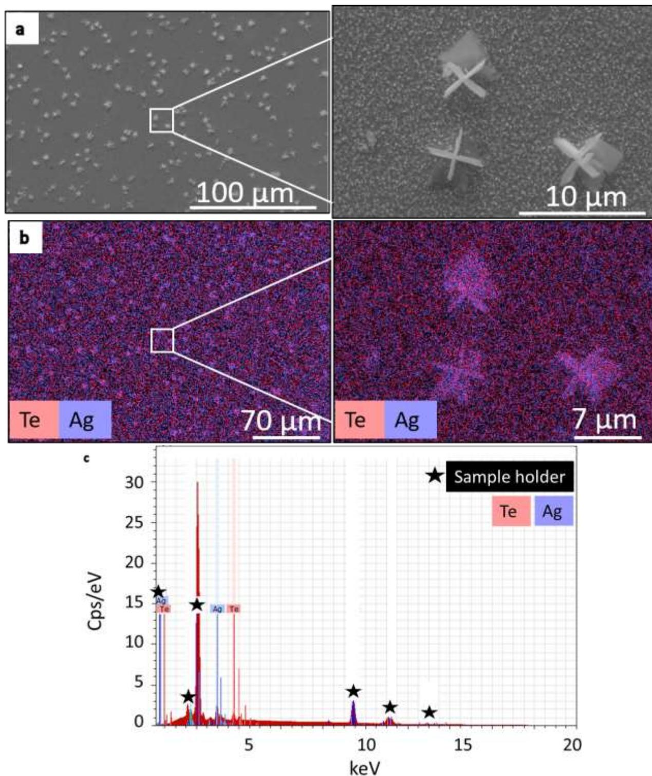
Fig. 7: SEM characterization of  $\text{Ag}_2\text{Te}$  nanorods film after 24h immersion prepared with  $n\text{Ag(I)}/n\text{Te} = 772$ : a) SEM image, b) EDX mapping, c) EDX spectrum.
