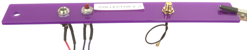
Fig. 8. Connector and tare button on the Base Front plate.
