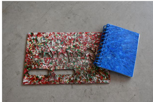
(c) Plastic sheet and notebook cover made from recycled material
