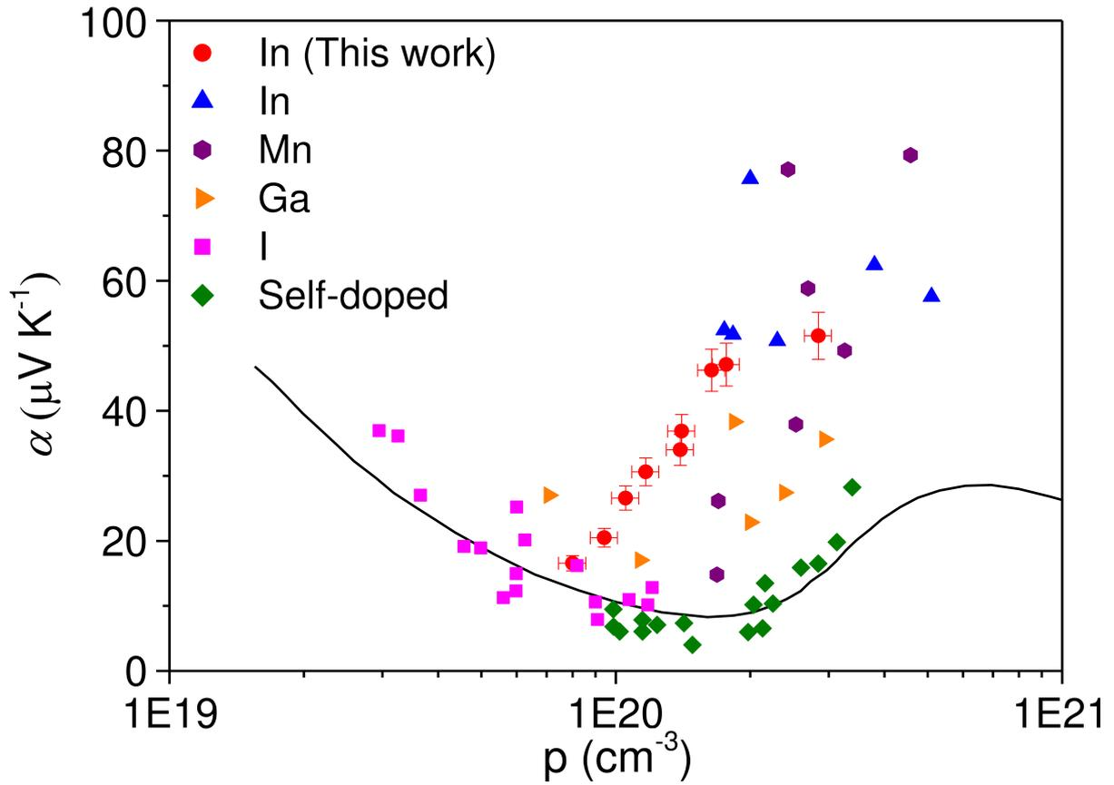
**Figure 1.** Ioffe-Pisarenko plot of SnTe showing variations in the thermopower  $\alpha$  as a function of the hole concentration  $p$ . The black solid curve stands for the theoretical dependence calculated using a two-valence-band model.<sup>11,21,23</sup> The experimental data points are taken from the literature for In-doped,<sup>11,14</sup> I-doped,<sup>21</sup> Mn-doped,<sup>27</sup> Ga-doped,<sup>28</sup> and self-doped (that is, by Sn vacancies)<sup>14,22,23</sup> SnTe samples.
