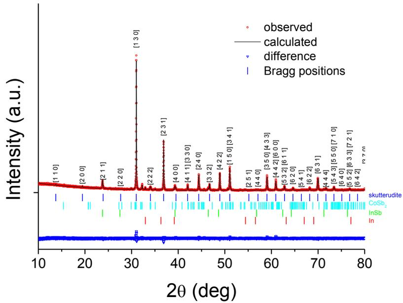
Fig. 2 XRD patterns of HPHT synthesized  $\text{InCo}_4\text{Sb}_{12}$ .
