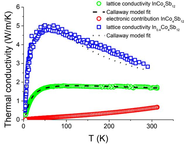
**Fig. 8** Temperature dependence of the thermal conductivity for  $\text{In}_{0.4}\text{Co}_4\text{Sb}_{12}$  and  $\text{InCo}_4\text{Sb}_{12}$  fitted with a Callaway model (more detailed description in the text).
