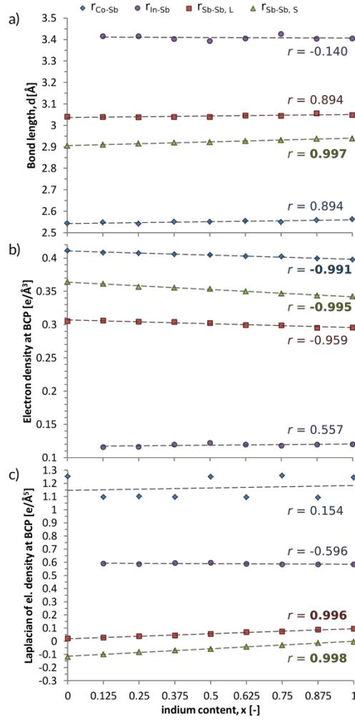
**Fig. 12** Average properties of total electron density at BCPs in  $\text{In}_x\text{Co}_4\text{Sb}_{12}$ : a) bond length [ $\text{\AA}$ ], b) electron density [ $\text{e \AA}^{-3}$ ], c) Laplacian of electron density [ $\text{e \AA}^{-5}$ ], in dependence of indium content. Dashed lines are added as a guide to eyes. Also, for each set of points calculated value of Pearson correlation coefficient  $r$  is given.
