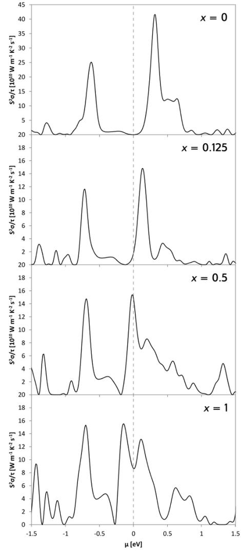
**Fig. 11** Seebeck coefficient ( $S$ ) and power factor ( $S^2\sigma$ ) reduced by relaxation time ( $\tau$ ) for  $\text{In}_x\text{Co}_4\text{Sb}_{12}$  with respect to chemical potential ( $\mu$ ) calculated at 300 K.
