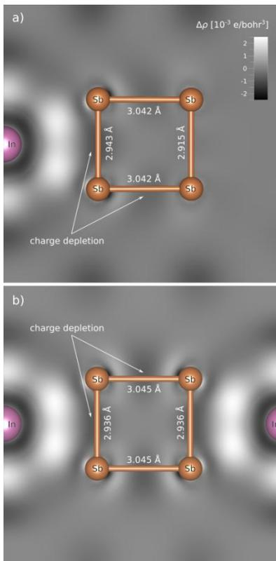
**Fig. 13** Differential charge density projected on  $Sb_4$  plane in  $In_{0.75}Co_4Sb_{12}$  structure. Differential charge density was calculated as a difference between electron density distribution in  $In_{0.75}Co_4Sb_{12}$  and a sum of separated In and  $CoSb_3$  structures, without changing atomic positions:  $\Delta\rho = \rho_{In_{0.75}Co_4Sb_{12}} - (\rho_{Co_4Sb_{12}} + \rho_{In_{0.75}})$ .
