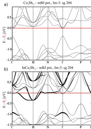
**Fig. 9** Band structures of undoped  $\text{CoSb}_3$  (a) and filled with indium  $\text{InCo}_4\text{Sb}_{12}$  (b), calculated using modified Becke-Johnson potential. In (b) indium character projected on every band is indicated by line thickness.
