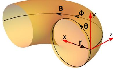
Figure 1: A tokamak (torus) transection, the external magnetic field  $\mathbf{B}$  (its dominant toroidal part), the toroidal coordinates  $(r, \theta, \Phi)$  where  $\mathbf{r}$  is the radius unit vector,  $\boldsymbol{\theta}$  and  $\boldsymbol{\Phi}$  are the poloidal and toroidal unit vectors; the introduced Cartesian coordinates in red  $(x, y, z)$
