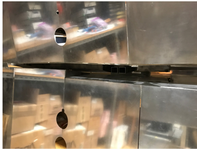
Figure 17. Mock-up of gap 4 provided by the IO featuring the relevant geometry of the first-wall surfaces and BMs surrounding the PPR antennas.
