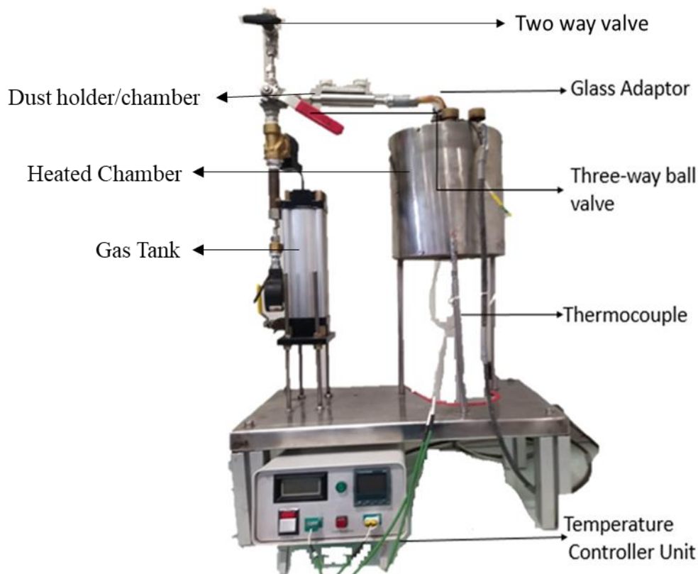
Figure 9: The Godbert-Greenwald (G-G) furnace
