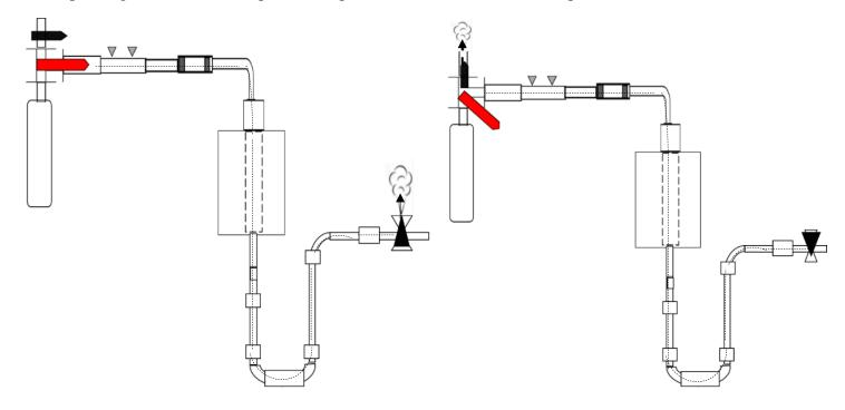
Figure 11: Powder dispersion/flash pyrolysis configuration to the left and Argon Flushing configuration to the right.
