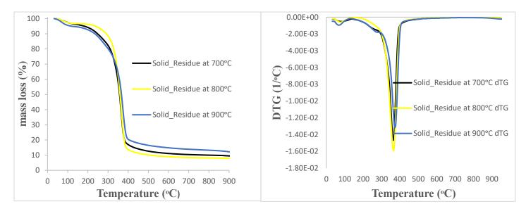
Figure 21: TG (left) and dTG (right) thermogram of cellulose solid residues
