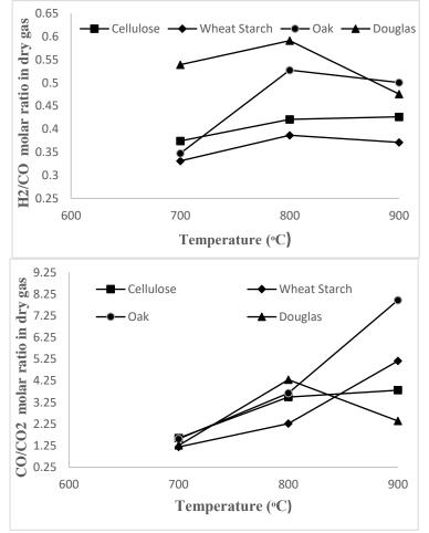
Figure 23: Effect of reactor temperature on H<sub>2</sub>/CO, CO/CO<sub>2</sub> molar ratios on dry gas compositions.
