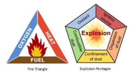
Figure 2: Dust explosion pentagon and fire triangle adapted from [5]
