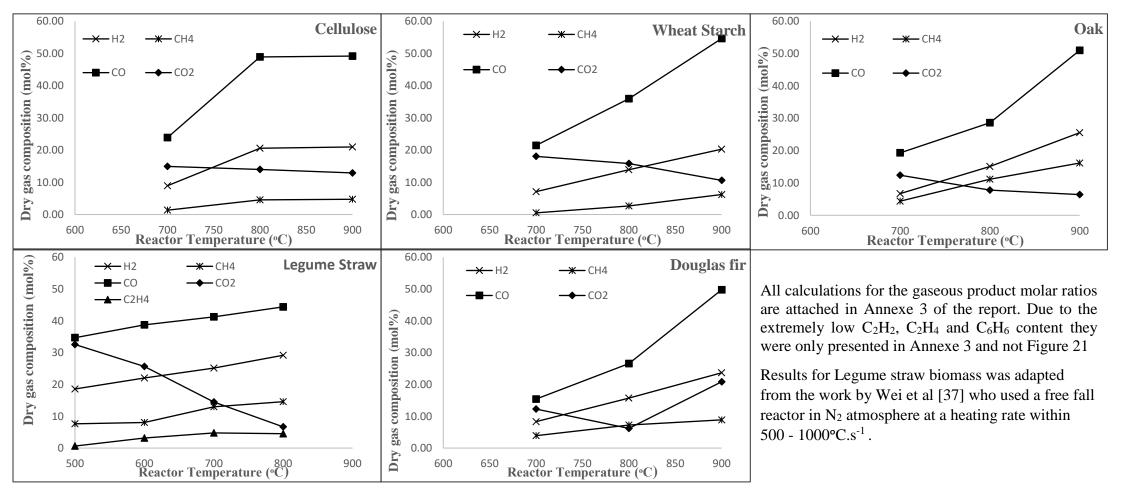
Figure 22: Effect of reactor temperature on dry gas compositions
