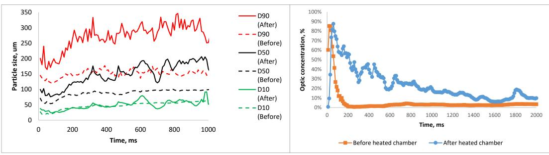
Figure 15:  $D_{10}$ ,  $D_{50}$ , and  $D_{90}$  Characteristics parameters of dispersed cellulose dust before and the heated furnace as a function of time
