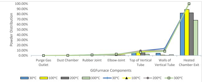
Figure 17: Organic dust segregation in the G—G furnace during dispersion
