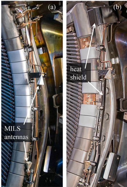
Fig. 4. MILS diagnostic in AUG with two horn antennas and microwave waveguides: (a) without the thermal shield, (b) with the thermal shield.
