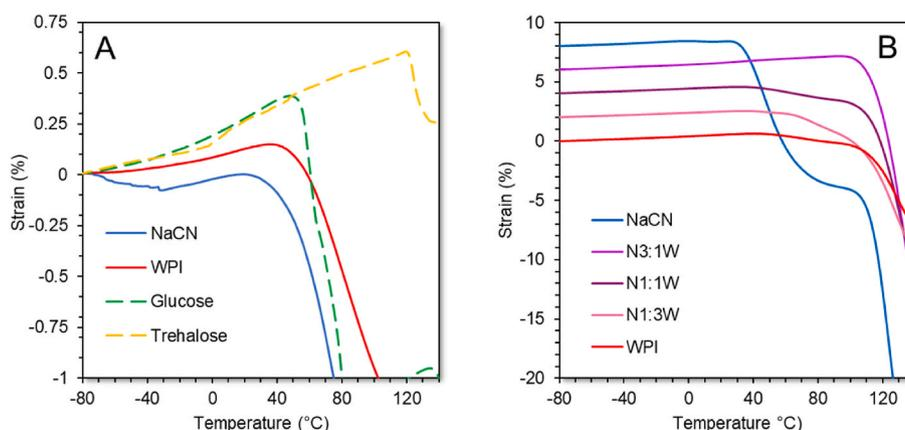
**Fig. 10.** Thermo-mechanical profile of individual ingredients of the cryogels (A) and milk protein cryogels (B). For improved readability, the TMA spectra of NaCN, N3:1W, N1:1W and N1:3W cryogels were shifted upward by 8, 6, 4 and 2%, respectively.
