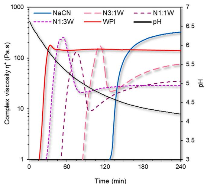
Fig. 1. Representative lactic acid-induced protein gelation profiles of the NaCN and WPI, as well as their blends determined by isothermal oscillatory rheology ( $f = 1 \text{ Hz}$ ,  $\gamma = 0.1\%$ ,  $37^\circ\text{C}$ ). The decline of pH throughout the fermentation is represented by the continuous black line.
