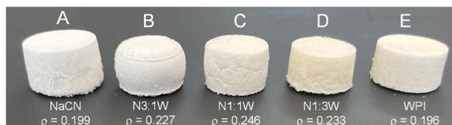
Fig. 4. Macroscopic appearance of the milk protein cryogel monoliths embedding LGG cells. The bulk density of the cryogels ( $\rho$ ,  $n = 8$ ) is expressed in  $\text{g}\cdot\text{cm}^{-3}$ . Approximative cryogel dimensions: diameter  $\times$  height = 15  $\times$  10 mm.
