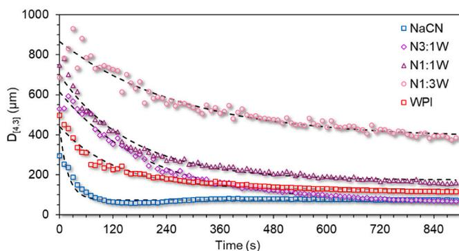
**Fig. 11.** Disintegration profile of the NaCN, WPI and blend cryogels measured at 20 °C and with a constant shear speed of 3500 rpm. Black lines represent the fitted data using the first-order exponential decay model (Eq. (4)). The curves and the points represents the average of 5 individual disintegration experiments.
