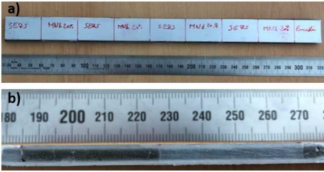
Fig. 4. a) Top view and b) side view of a sandwich composite with a 4 cells periodic structure
