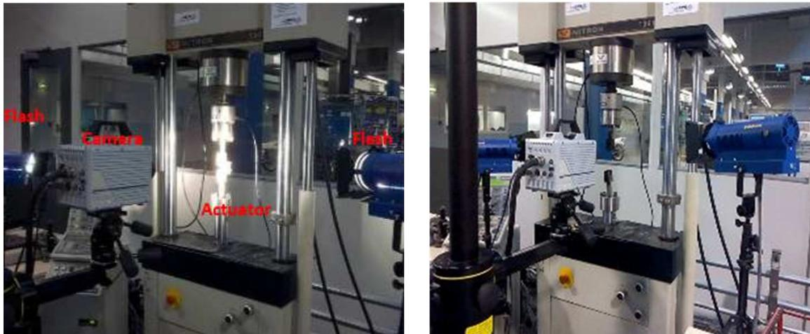
**Fig. 18: Experimental test set-up**
