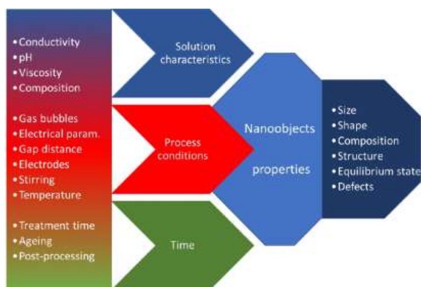
Fig. 3 Links between process parameters and nanoobjects properties
