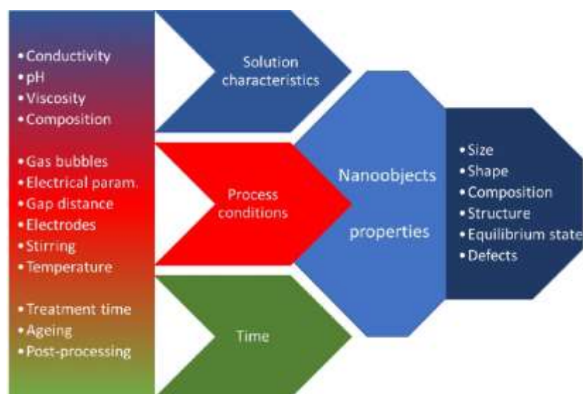
Fig. 3 Links between process parameters and nanoobjects properties
