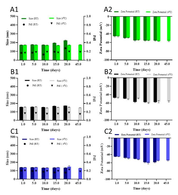
**Figure 2**: Hydrodynamic diameter ( $d_H$ ) and PdI of LDC 1 (A1), 2 (B1) and 3 NPs (C1), at room temperature (RT) or 4 °C over time. Zeta potential (mV) of LDC 1 (A2), 2 (B2), and 3 NPs (C2), at room temperature (RT) or 4 °C over time.
