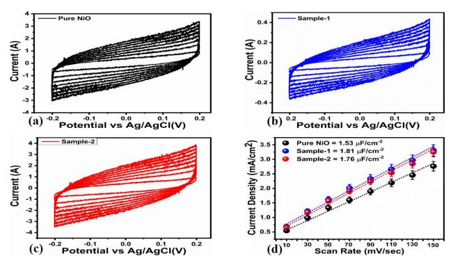
**Figure —7.** (a–c) CV curves measured at non-Faradic region at various scan rates such as 10, 30, 50, 70, 90, 110, 130, and 150 mV/s in 0.1 mM urea for pure NiO and sample 1 and sample 2, (d) linear plot of current density against different scan rates for the calculation of ECSA.
