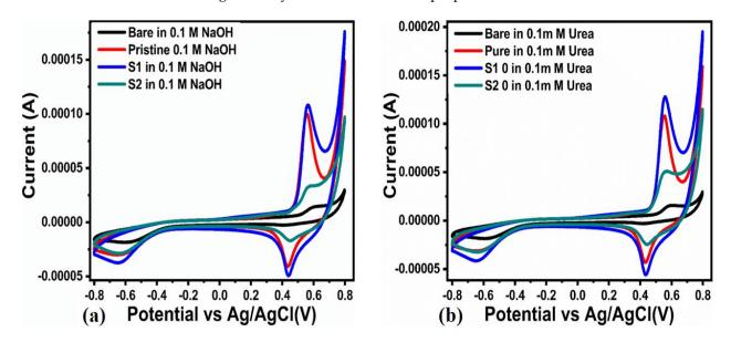
**Figure -2.** (a) Cyclic voltammogram of bare GCE and MGCE with pristine NiO and sample 1 and sample 2 of NiO nanostructures prepared with 10 mL and 15 mL of bitter gourd peel extract at 50 mV/s in 0.1 M NaOH, (b) cyclic voltammogram of bare GCE and MGCE with pristine NiO and sample 1 and sample 2 of NiO nanostructures prepared with 10 mL and 15 mL of bitter gourd peel extract at 50 mV/s in 0.1 mM urea.
