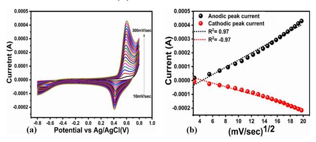
**Figure —3.** (a) Cyclic voltammogram of sample 1 prepared with 10 mL of bitter gourd peel extract at various scan rates in 0. 1 mM urea, (b) linear plot of anodic and cathodic peak current against square root of scan rate.
