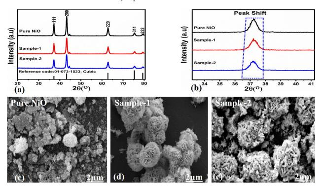
Figure —1. (a) X-rays fiffraction patterns of NiO nanostructures prepared with 10 mL, 15 mL, and without the bitter gourd peel extract, (b) the shift in the two-theta angle, (c) SEM image of pure NiO, (d) SEM image of NiO nanostructures prepared with 10 mL of bitter gourd peel extract, (e) SEM image of NiO nanostructures with 15 mL of bitter gourd peel extract.
