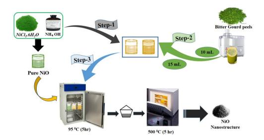
**Scheme 1.** Representation of phytochemical synthesis of NiO nanostructures using bitter gourd peel extract.
