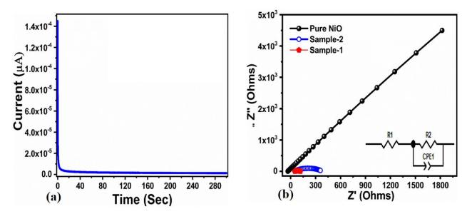
**Figure —6.** (a) Stability measurement using chronoamperometry at 0.5 V for 300 s in the presence of 0.1 mM urea, (b) fitted Nyquist plots for pure NiO and sample 1 and sample 2 measured at 100 kHz to 0.1 Hz, sinusoidal potential of 10 mV and biasing potential of 0.5 V in 0.1 mM urea.
