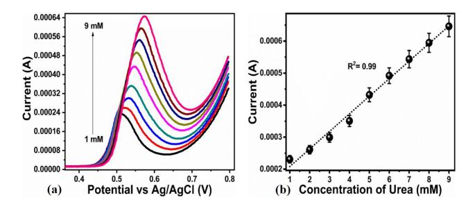
**Figure -4.** (a) Cyclic voltammogram of sample 1 prepared with 10 mL of bitter gourd peel extract at v50 mV/s in various urea concentrations ranging from 1–9 mM, (b) linear plot of peak current versus urea concentrations.
