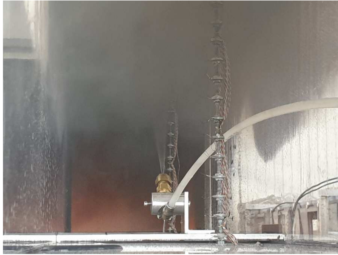
Figure 4: Rear view from the exit of an upward water spray with a 45° angle
