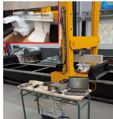
Fig. 6. Measurement setup during bending tests. Inset: mounting configuration of the interrogation antennas.
